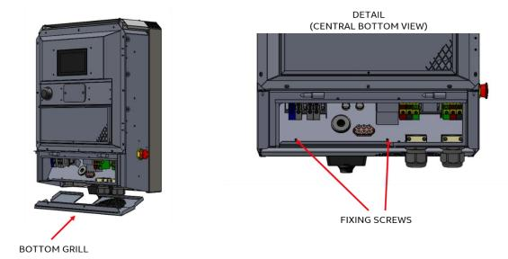
10. Take the lower frontal cover and place it on the lower side of the unit. Secure it in place by tightening the two screws.
