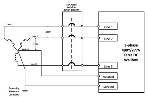
Electrical grid configuration required for 3-phase, DC Wallbox UL variant (3ø, 480Y/277V input)
