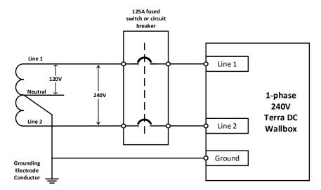
One of two electrical grid configurations acceptable for use with 1-phase, DC Wallbox UL variant (1ø, 240V input)
