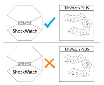
Checking the Shock Watch and Tilt Watch PLUS sensors:
