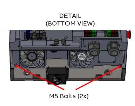
7. Let the auxiliary power supply cable pass through the central gland and tighten it.
