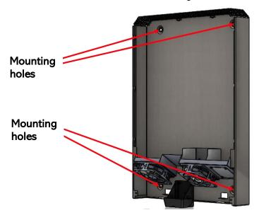
5. Place the unit on the wall frame by correctly aligning the 6 bolts (3 for each lateral side).
