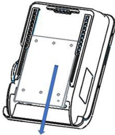
Figure 1-5 Remove the mounting bracket
