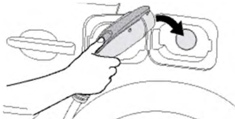
Figure 5-3 Connect the charging plug to the EV
