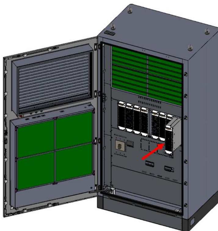
Figure 36 Installation of the power module
