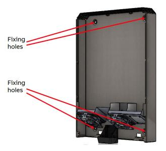
5. Put the unit on the cabinet correctly aligning the 6 bolts (3 for each lateral side) between them.
