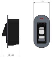
Figure 4: Terra DC wallbox optional Gun holder; front and side view.
