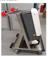
7. When desired location is reached, put the brakes of each castor, this will keep the cart from rolling away when you want it to stay put.
