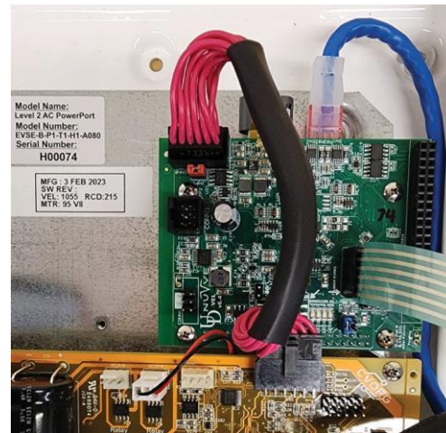
Figure 3b. RJ45 cable connected to the internet port of the red circuit board (Built Version 2.2, Green board Version 6.4)
