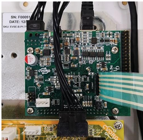
Figure 3a. RJ45 cable connected to the internet port of the red circuit board (Built Version 2.1, Green board Version 5.3C)
