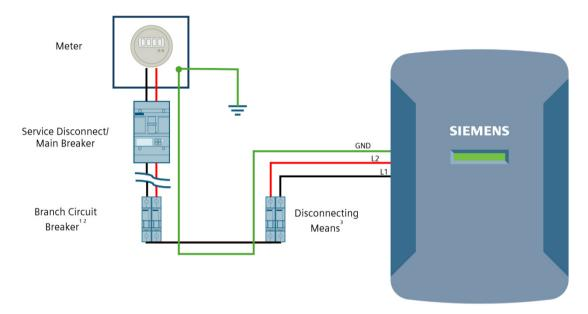
$<sup>^{1}</sup>$  Branch circuit shall be rated ≥125% of the current setting of the EVSE. Consult Sections 625.41 and 625.42 of the NEC for detailed information.
