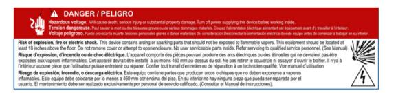
This label indicates the risk of hazardous voltage and electric shock which will cause death, serious injury or substantial damage. Turn off the power supplying this VersiCharge before working inside.
