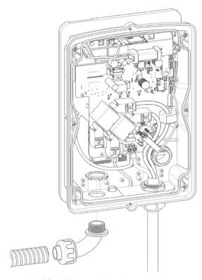
Install 1" flexible conduit and NPT connector per the manufacturer's installation instructions
