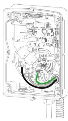
1. Route the wires into the enclosure.
