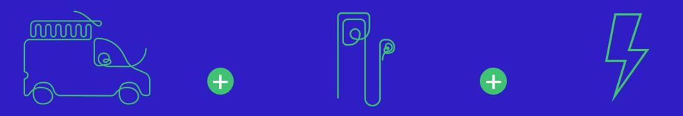
Analysis of the vehicle's energy requirements according to the distance (mi) to be covered Identification of charging opportunities (periods when the vehicle is parked) Calculation of the power required for each charge to guarantee sufficient energy for vehicle operation
