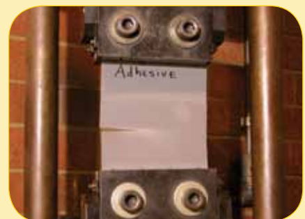
D ADHESIVE AFTER: Adhesive after pull test. Adhesive at 2" overlap, metal tears at an average of 13,260 lbs. (joint did not break).
