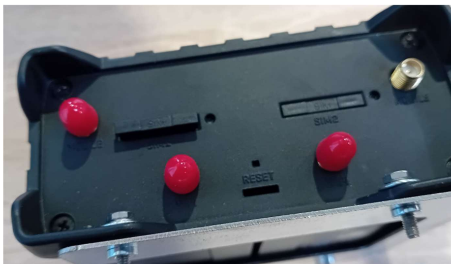
Figure 54 View of the sim card holder extended
