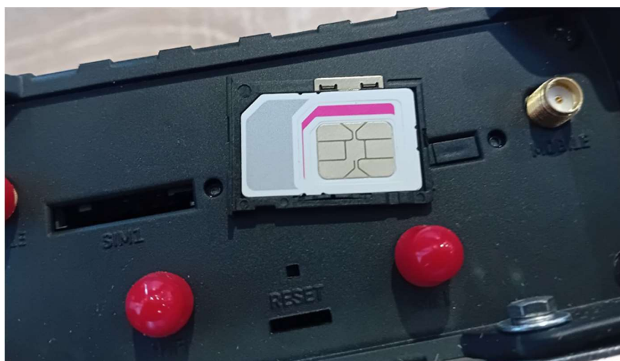
Figure 55 Correctly placed sim card in the holder
