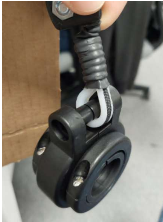
Figure 30 Mounting the CCS cable holder to the balancer
